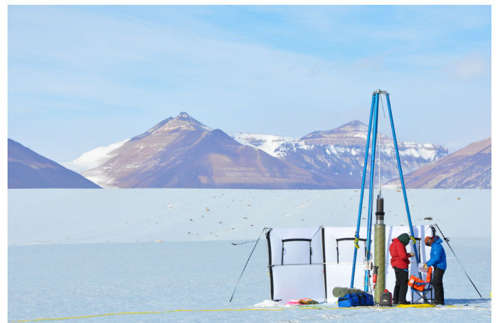
Drillers with the Blue Ice Drill at Taylor Glacier, Antarctica. Photo: Jeff Severinghaus
