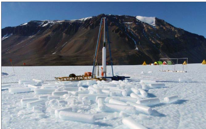
The Blue Ice Drill is designed to collect large volumes of ice (9.5-inch diameter cores) in a short period of time. The large volumes of ice enable ultra-trace gas measurements, such as the carbon-14 of methane, that historically have been precluded by sample size limitations of ice cores. Photo courtesy of Tanner Kuhl.
